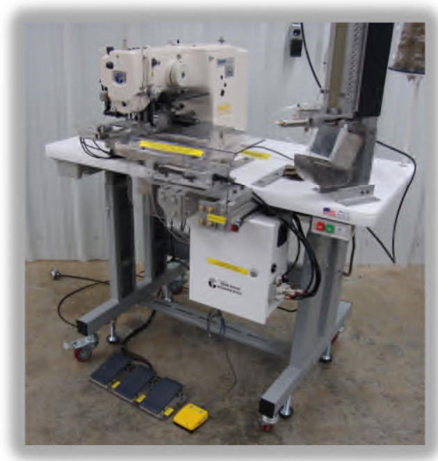
CEDAR Systems CS-1306 & ODC-2512 Electronic, Programmable Pattern Machine With "On Demand" Cold Cut Device
