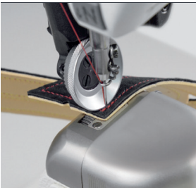
Single-needle lockstitch post-bed stepping roller feed machine (left-hand/right-hand) with large vertical rotary hook
