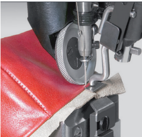
Single-needle lockstitch post-bed roller feed machine (right-hand) with large vertical rotary hook
