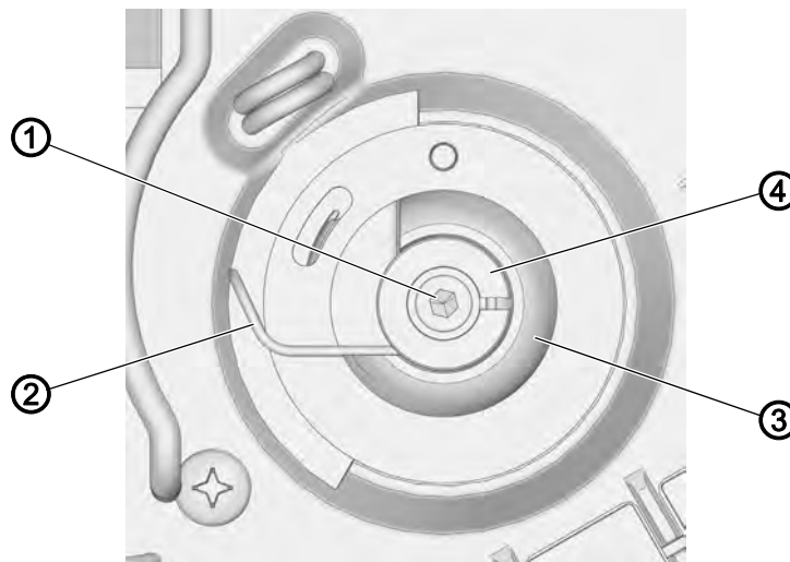
Fig. 54: Setting the thread tension spring
