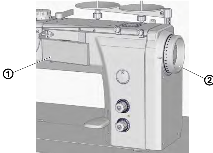
Fig. 23: Setting the reference position of the handwheel
