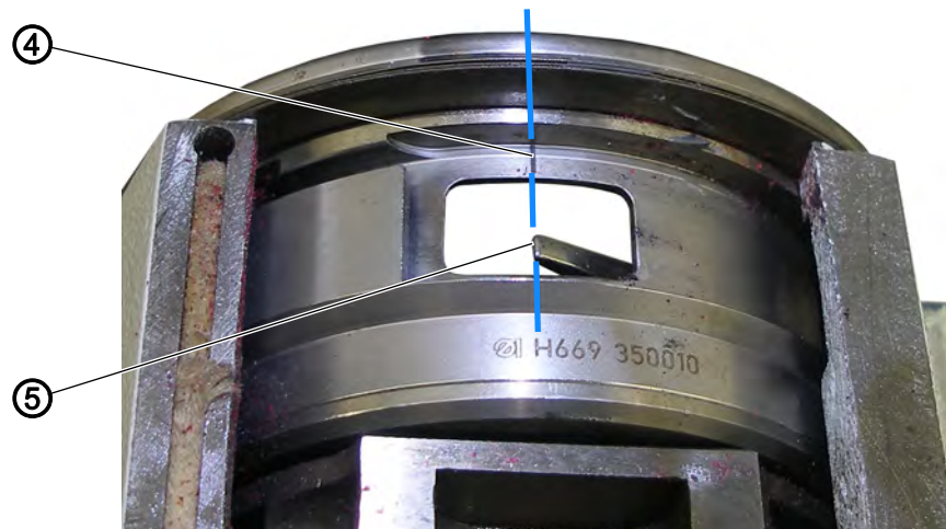
Fig. 42: Setting the dead center of the reciprocating hook movement (3)
